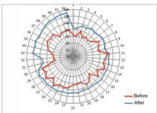
In a 175 TPD kraft machine in Egypt, the dryer surface temperatures varied between 60 and 80 deg C.
