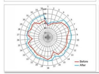
At a 140 TPD kraft unit in Vapi, Forbes Marshall FBS rotary joints and syphons increased the average dryer surface temperatures by 25 deg C. Now the machine is operating with a differential temperature of 27 deg C between steam and dryer surface.
