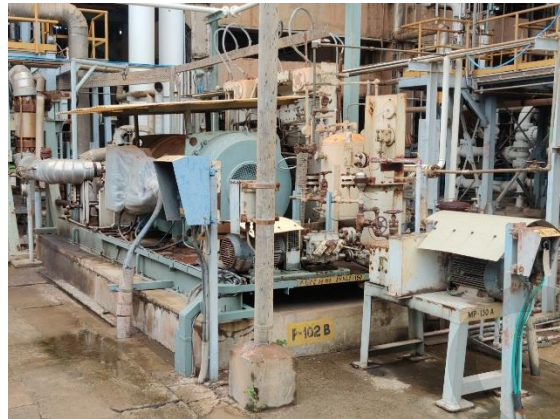
Figure 3.10: Urea 1 P-102B Pump & Motor
