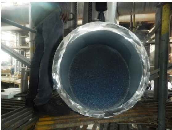
Figure 3.11: Equipment Choked with Catalyst
