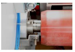
The treater ground rolls are dynamically balanced and has an electronic zero speed switch and grounding brush to prevent premature bearing failure. The Treater rollers will be of approximately 120mm Diameter with Silicon Sleeves.
