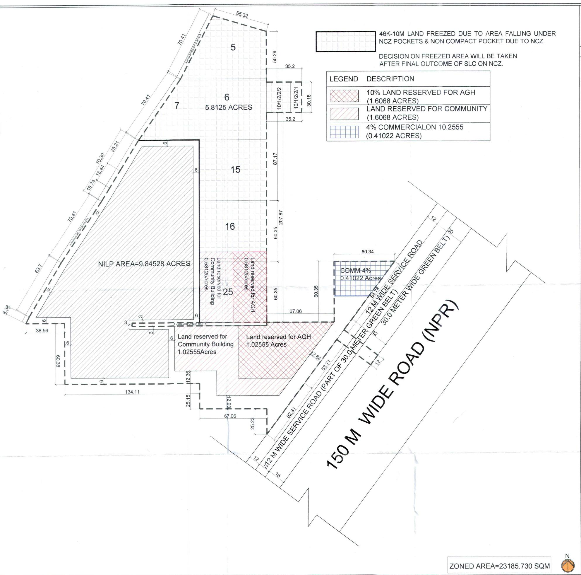
ZONING PLAN FOR RESIDENTIAL COLONY UNDER NILP POLICY -2016 ON THE AREA MEASURING 10.30 (AFTER FREEZING OF AN AREA MEASURING 5.8125 ACRES (46K-10M) FALLING UNDER NCZ AND NON COMPACT POCKET DUE TO NCZ) (LICENCE NO. 1.06. OF 2022, DATED ....518.12022.... AT SECTOR-113 DISTRICT GURUGRAM, HARYANA BEING DEVELOPED NOURISH DEVELOPERS PVT. LTD
