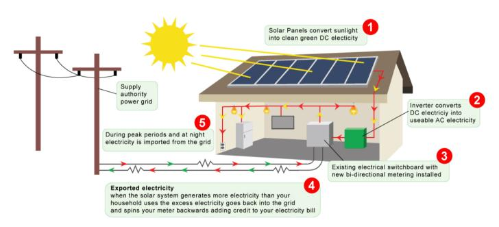
Operating silently and without any moving parts or environmental emissions, PV systems have developed from being niche market applications into a mature technology used for mainstream electricity generation. A Rooftop/Ground system recoups the invested energy for its manufacturing and installation within 0.7 to 2 years and produces about 95 percent of net clean renewable energy over a 25-year service lifetime
