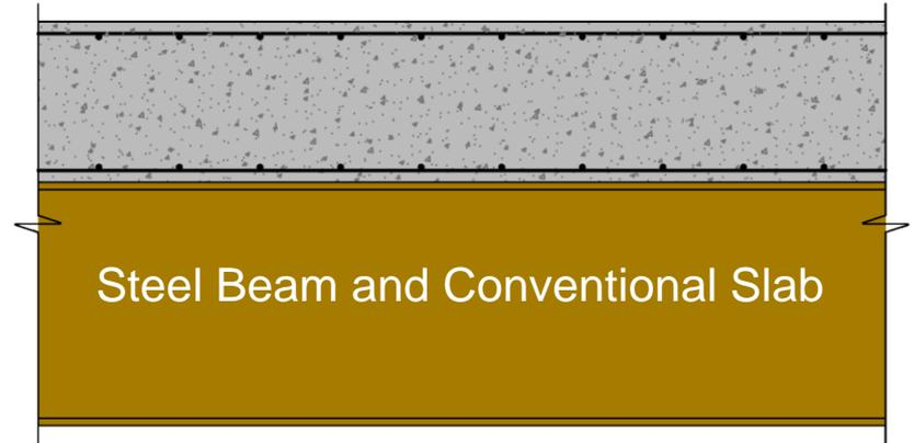
(based on 130mm deep composite metal deck slab / 300mm deep flat RC slab)
