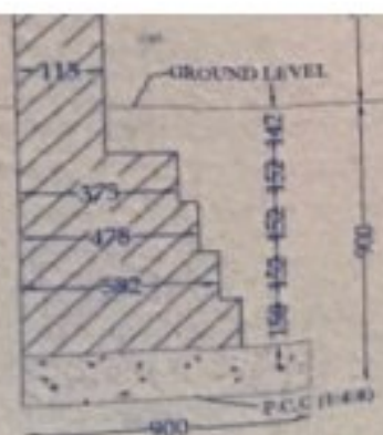
BOUNDARY WALL SCALE 1:20
