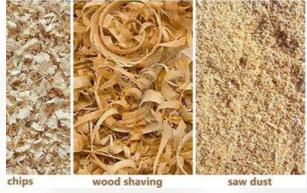
Industrial waste: This includes sawdust, wood shavings, and other wood residues generated from wood processing industries.
