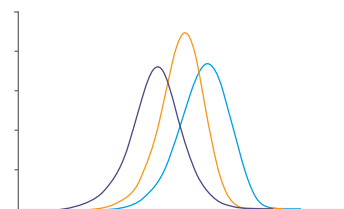
Molecular weight distributions for three polyethylene samples – purple plot shows the unbranched sample.
