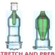
STRETCH AND PREBLOW BIAXIALLY ORIENTED HIGHLY STRESSED STRUCTURE
