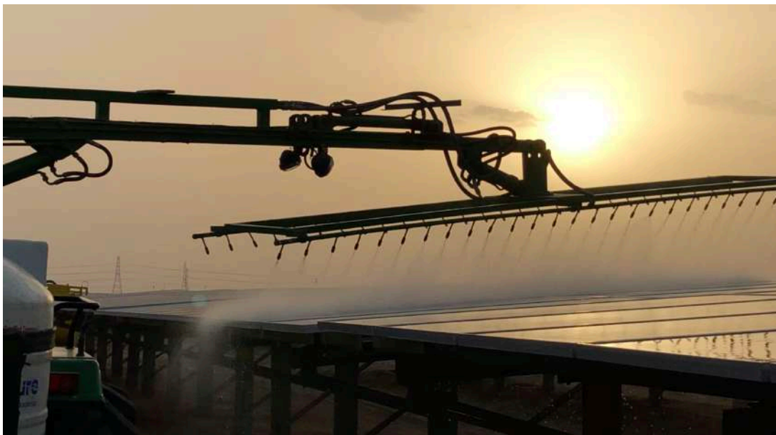
In-house designed Trac-Robots for washing modules resulting in high efficiency
