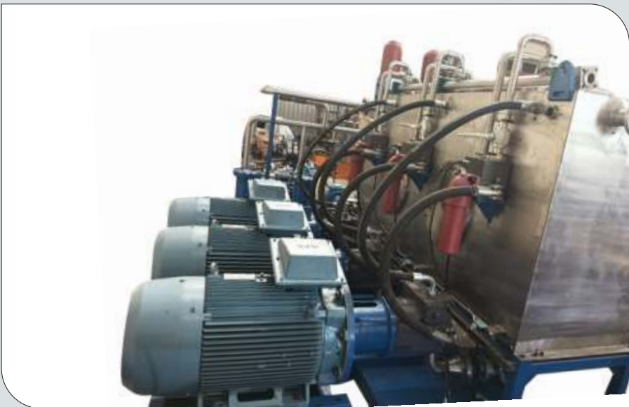
Hydraulic Power Pack for AGC
