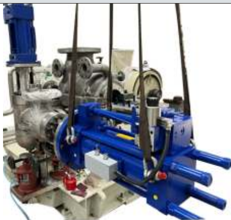
Control Valve Actuator for Steam Turbine
