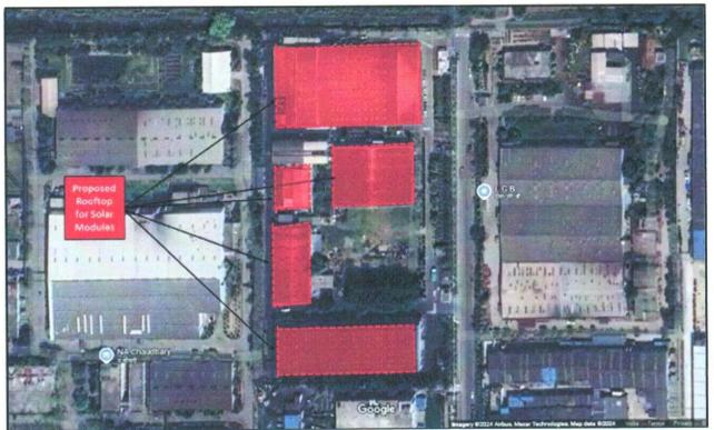
Based on analysis using Google's imagery tool, no significant shadows or obstructions were detected on the roof that could block direct sunlight.
